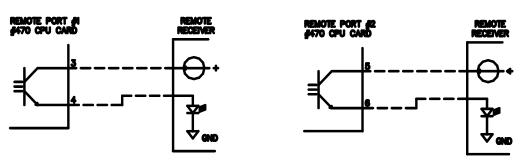
20mA "PASSIVE" CURRENT LOOP CONNECTIONS
