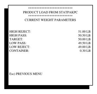
The operator cannot access or change these parameters, only view them. To make changes to weight parameters, the operator must make these changes directly in the StatPak-PC software.
