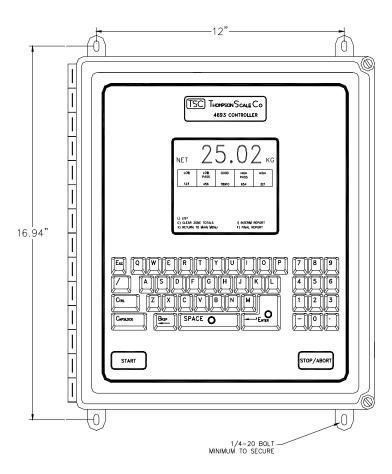
The Checkweigher controller cabinet is a Nema 4X rated fiberglass or optional Stainless Steel enclosure. Overall Size is 16" x 14" x 8" in depth, with S.S. hinge and cover screws. The front panel of the controller is overlaid with a membrane switch panel which also contains a 4.3" x 5" scratch resistant display window. Mounting feet are provided for wall or plate mounting.
