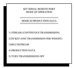
Select item #4 "Production Data". This enables the down-time logging feature, and performs two (2) functions.
