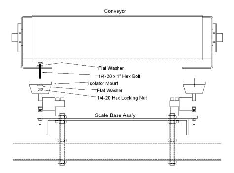
Once the conveyor is in place and secured, the support stand can be placed into the conveyor line, and the leveling feet used to ensure that the conveyor is level in both length and width, and that the conveyor height matches the in-feed and out-feed conveyors.
