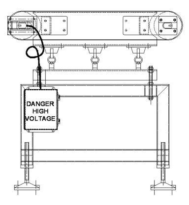
The motor leads from the motorized pulley should include a service loop between the end of the pulley and the connector on the junction box or motor control enclosure. This service loop provides a flexible connection, allowing the scale to move freely.
