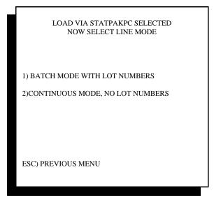
If your application produces the same packaged material on a continuous basis, such as 50 lb bags of plastic pellets, and lot numbers are never assigned to the production runs, then this line would be considered as a continuous production line.
